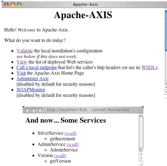
Fig. 13.8. The screen shot on the top shows the Axis home page, giving a list of utilities. The bottom shot shows the list of the deployed Web services, including the SilverService just deployed.
